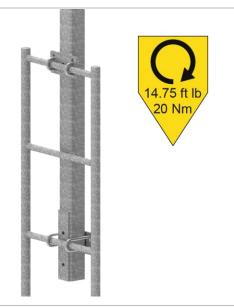
Evenly tighten the nuts to a torque of 14.75 ft lb (20 Nm).
